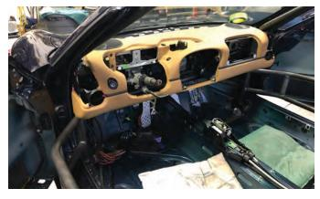
Dash fully fitted and installed
