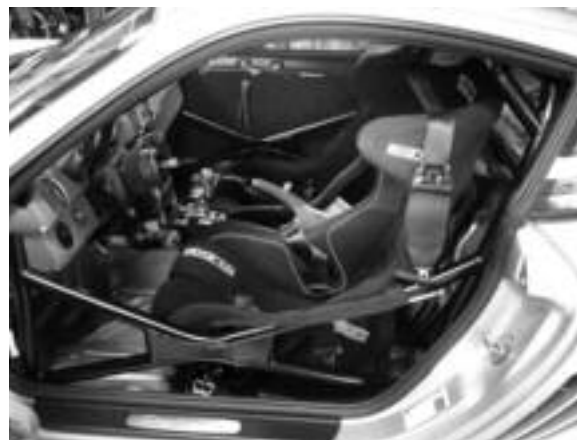
Above: The full cage that Vrankovich had installed by Piper Motorsports. By removing the inner door panels, Piper was able to place the cage's door bars farther from the driver, an important safety consideration.
