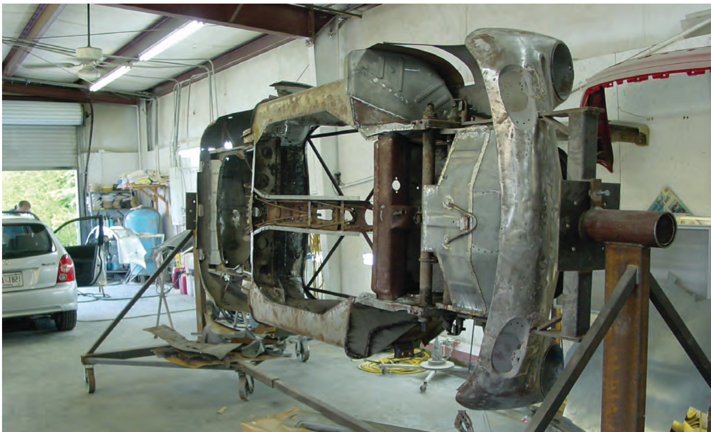
Body work commenced in 2003 on a rotisserie jig at Automotivation in Calhoun, Georgia. Note rusted body pans have been removed prior to fabrication and installation of new ones. Photo courtesy of Karl Milliren.
