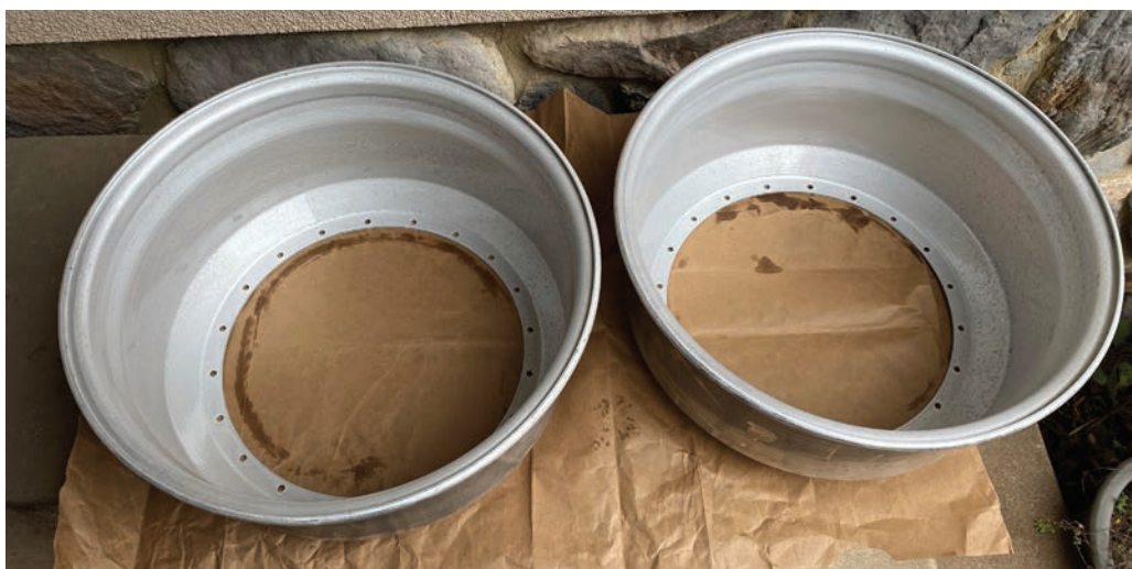
After flushing the barrels with water and applying two coats of Sharkhide Metal Protectant, the inner barrels looked acceptable
