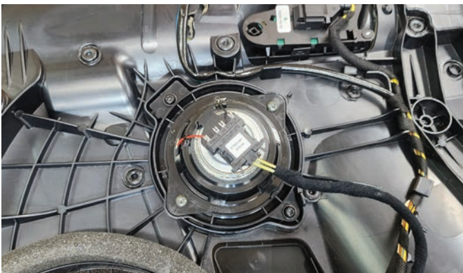
Upgraded 3" midrange on custom mount on backside of door panel.
