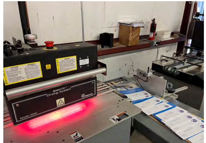
Your addresses were printed individually on the rear cover of each magazine at this inkjet labeling station run by Heidi Violette
