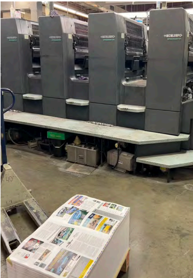
Our monthly magazines are printed on a Heidelberg Press that can print more than 10,000 sheets/ hour
