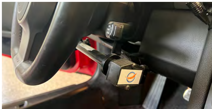
The accelerator potentiometer is at the right-hand end of the control bar
