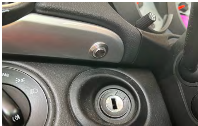
The hand control switchover button is located above the key slot
