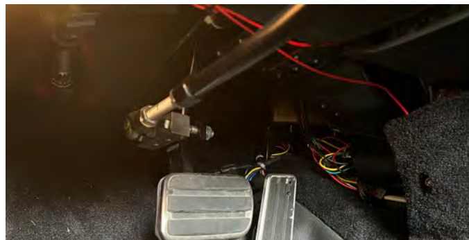
The hand control lever bolts directly to the brake pedal
