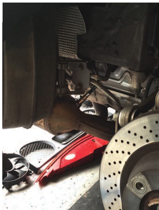
Below: The O2 sensor can be seen center of image.
