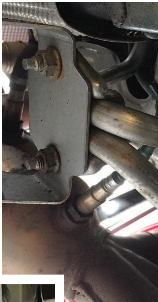
Left: The O2 sensor plugs into the exhaust before the cat converter (another view is below).
