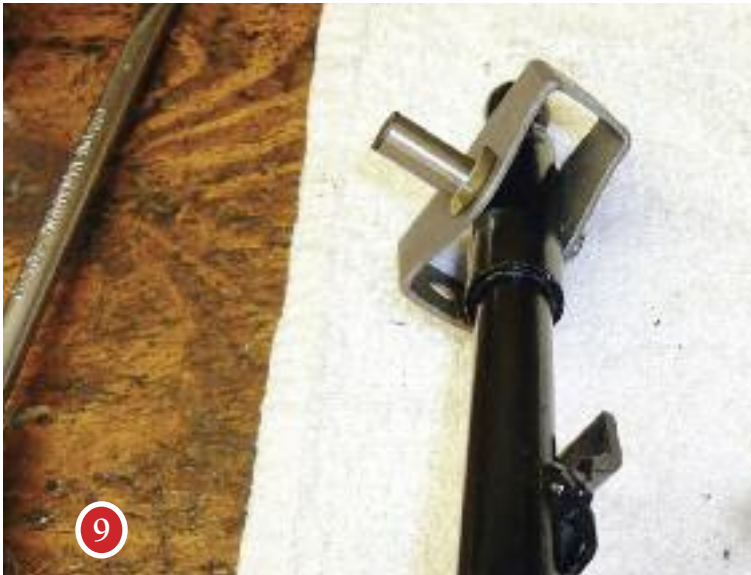
Insert the new pin, make sure the extended side is to the left.
