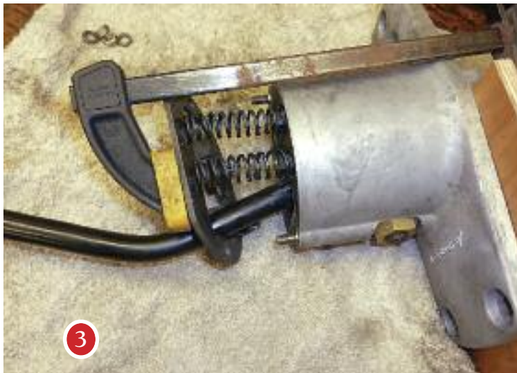
3 With the top plate removed, the old springs will come out. Now loosen the nut and remove the set screw.
