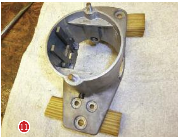
Insert the spring plate.
