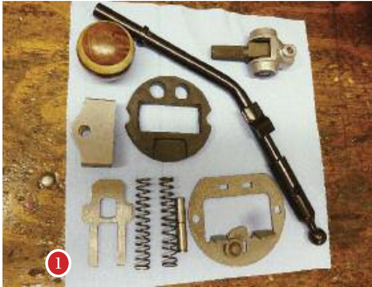
1 The necessary new parts, including the linkage with new bushings.
