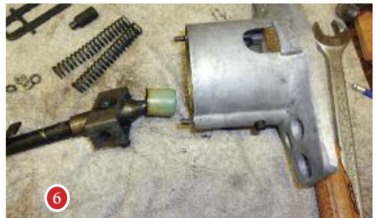
6 Now remove the shift rod and the piece that connects the whole thing.
