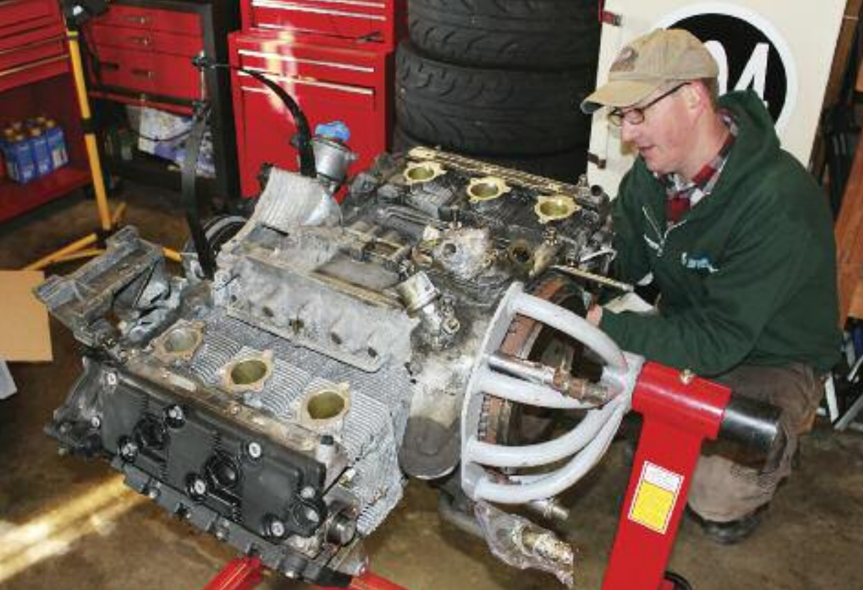
Photo by John Vrankovich Potomac member and DE enthusiast Don Mattingley works at disassembling the 3.6 liter engine from his 993. This was his first engine rebuild project, and he did most of the work himself with the help of a few friends.
