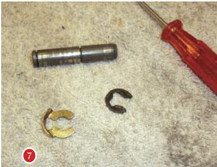
Remove the clips from the pin that lifts up the spring plate for 5th and reverse gear. They are needed for the new kit.
