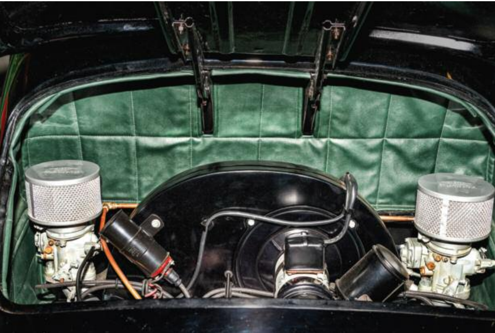
The engine compartment of the recently restored 1951 356 split-window coupe belonging to Pete Archibald. Photo by Ken Marks.
