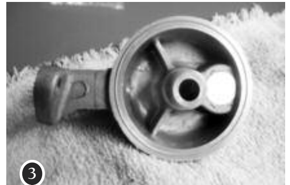
Figure 1: Earle's sandwich adapter with thermostat mounted on intermediate flange
