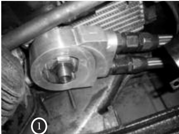
Figure 1: Earle's sandwich adapter with thermostat mounted on intermediate flange
