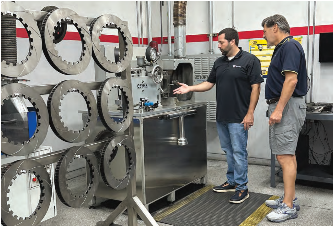
Matt Volk, sales manager at Essex, showing me one of their burnishing machines and a bunch of discs on the cooling rack.
