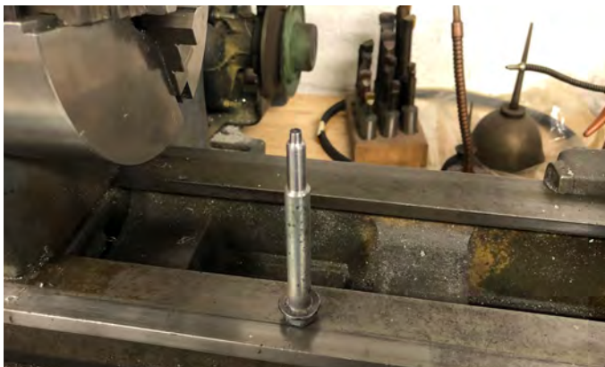
The bolt was turned on the lathe to become a custom tool for de-pinning the large connectors in the trunk
