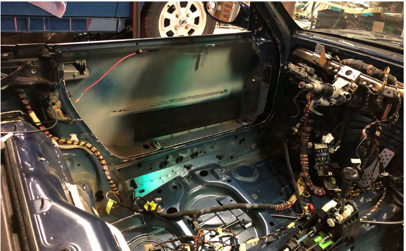
The start of trimming down the wiring harness. Would soon end up looking like the world's worst, bad-hair day
