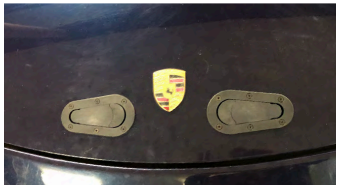
The front AeroCatch hood latches installed
