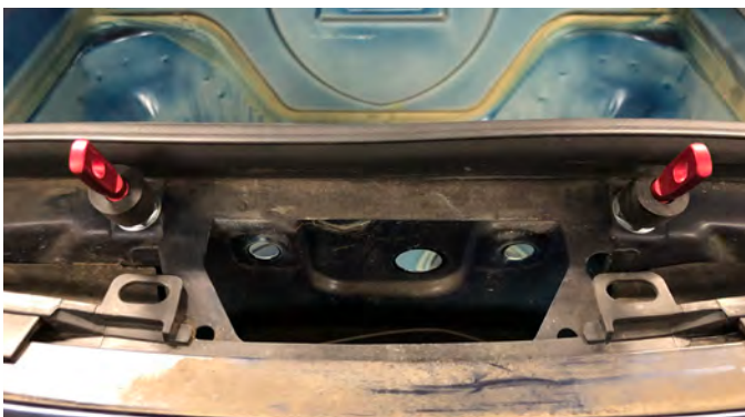
Installing the front AeroCatch hood latches. I first figured out where I wanted to install the pins — wanted to mount them outside the hood seal so that water would drain instead of accumulate inside frunk when it rains
