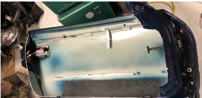
Door after gutting — just a bit of weight removed, and a new custom-made interior release handle
