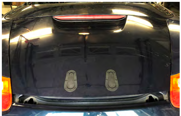
Matching rear AeroCatches installed. Couldn't fit them outside the hood seal, so still need to figure out how to seal the trunk from rain
