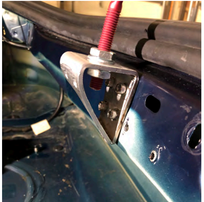
The rear AeroCatches took a little longer because I had to make custom brackets for the inside pins. Plus, there was no way I was going to fit inside
