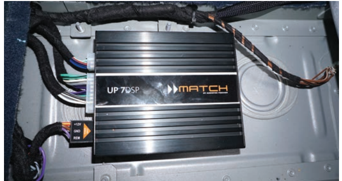
Amplified DSP installed in stock location under the passenger seat.
