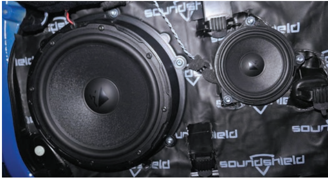
Replacement woofer and midrange on custom mounts with sound damping applied.
