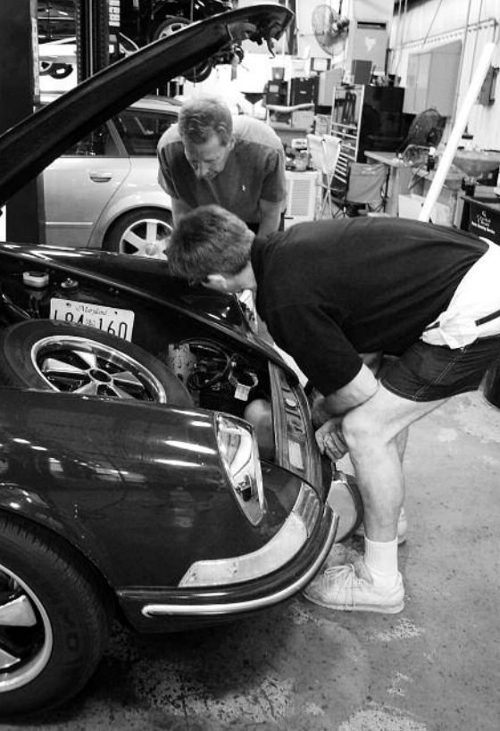
Above: Tech inspector and Club Historian George Whitmore, discusses a loose battery shield in John Hallen's '69 911 Targa. This model has twin batteries, one 6-volt battery in each fender of the front compartment.
