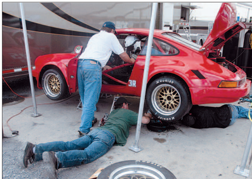
Above: Between session maintenance, bleeding the brakes at Summit Point's Shenandoah Circuit during a Driver Education event. The day saw temperatures in the 90s, so awnings or pop-ups were much in evidence.
