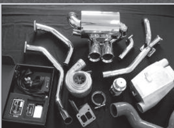
Cayman S & Boxster S turbo kit bolt-on 486hp
