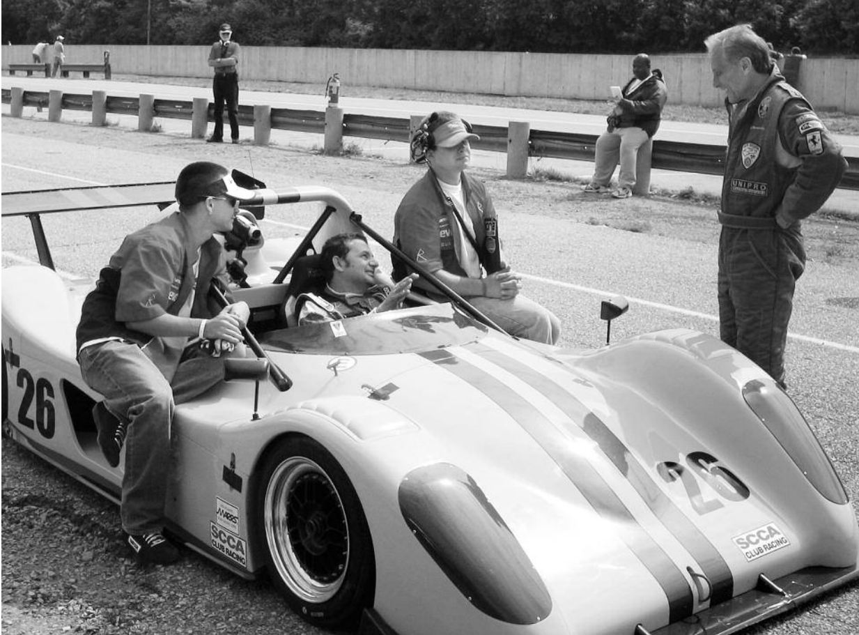
Photos by FunKtion Auto FunKtion auto owner Walid Ashi at the wheel of his Radical sports racer, powered by a Suzuki Hayabusa motorcycle engine, which he races at SCCA MAARS events.
