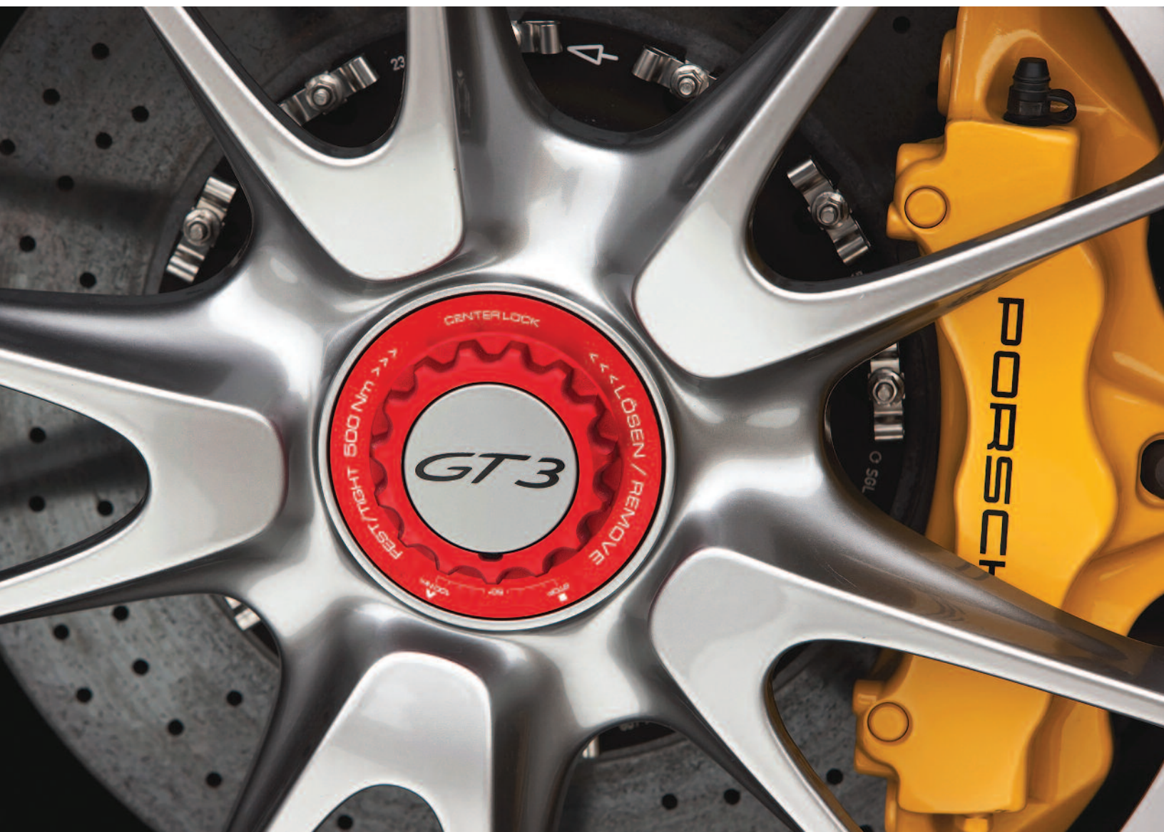
A 19-inch centerlock wheel for a new GT3 whose wheel bolts are in forged aluminum and finished in red epoxy plating. Photo provided by PCNA
