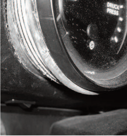
The gauge is held in place by a rubber gasket. Before replacing the gauge, coat the gasket with silicon paste.
