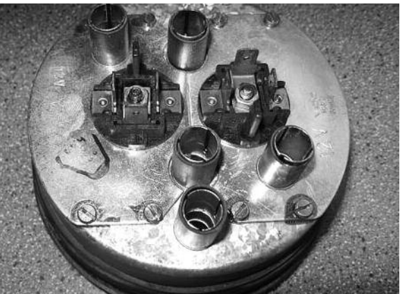
Remove the small screws that secure the temperature gauge panel
