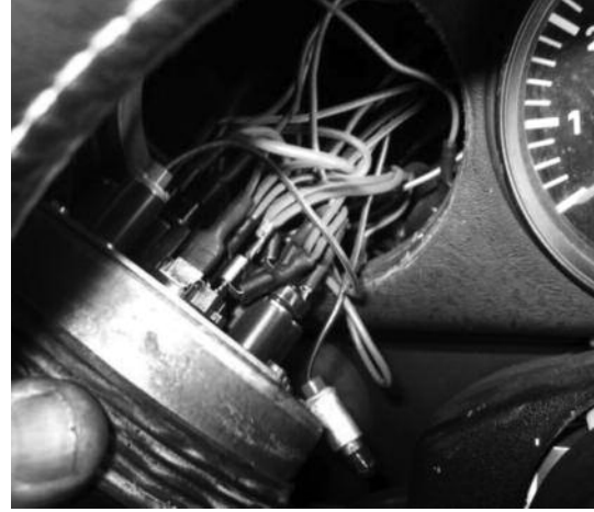
After removing the cluster from the dash, make careful note of placement of all wires and panel lights.
