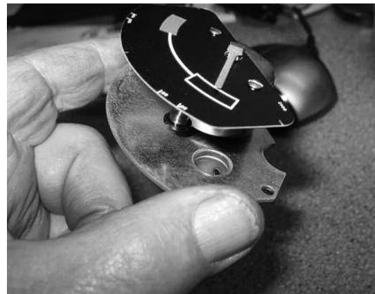
Be extra careful when removing the needle (Tip: use two teaspoons, one on each side of the needle, to pry it off gently).
