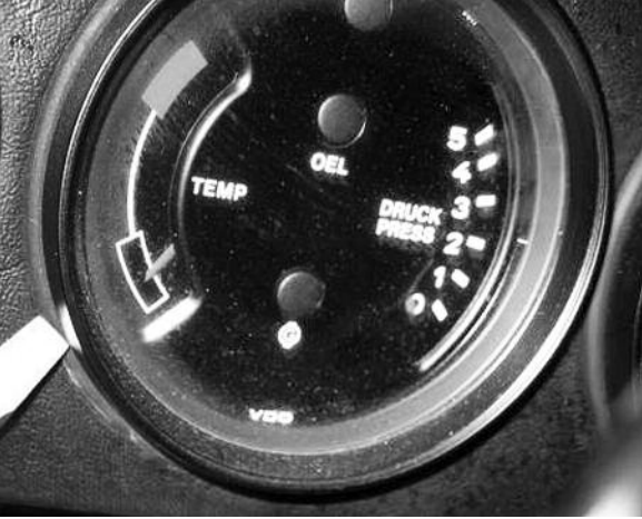
Original oil temperature gauge with the non-numbers face. Use screwdriver to pry the gauge cluster gently from the dash.
