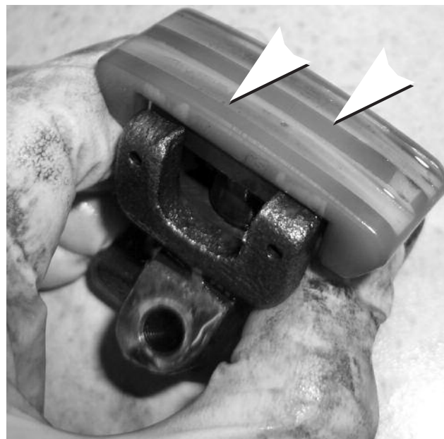
The tensioner after removal from the engine. Notice the obvious wear patterns (arrows).
