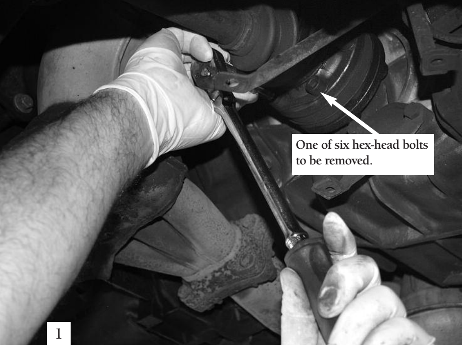
No. 1: Chapman loosens the six hex-head bolts first with a ratchet, then removes them with an air ratchet to save time. It's important to leave the car out of gear in order to rotate the axle to access all six bolts.
