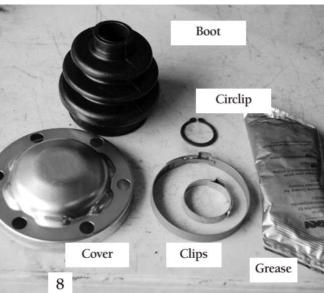
No. 6: A small clip secures the boot to the axle. Cut it off; a new one is in the kit.
