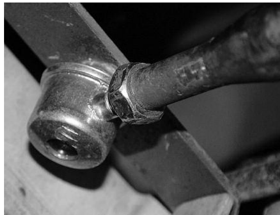
Left, below: The new angular joint (No. 16 in diagram) after installation. You'll need large pliers or C-clamp to squeeze the angular joint onto the ball.
