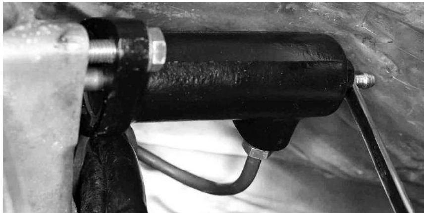
16 The new clutch slave cylinder attached to the bell housing.
