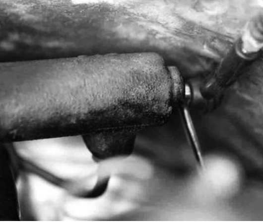
3 This is the view of the clutch slave cylinder from beneath the car showing the Vacula tool connected to the bleed screw at right.
