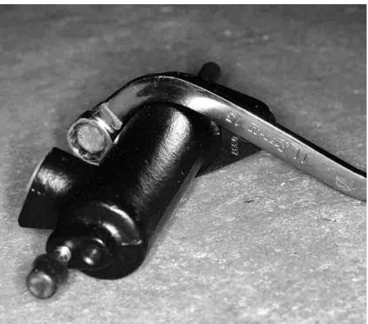
6 An "S" wrench makes removal of the upper 8mm bolt easy.
