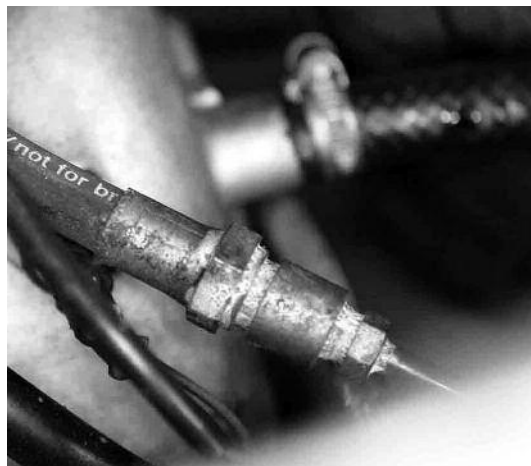
7 Remove the flexible line using both a 19mm and 12mm line wrenches.
