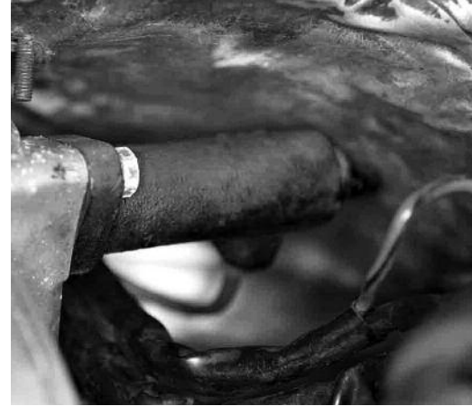
5 Remove the clutch slave cylinder by unfastening the two 8mm bolts and the 12mm ATF tube nut on the metal hydraulic line.
