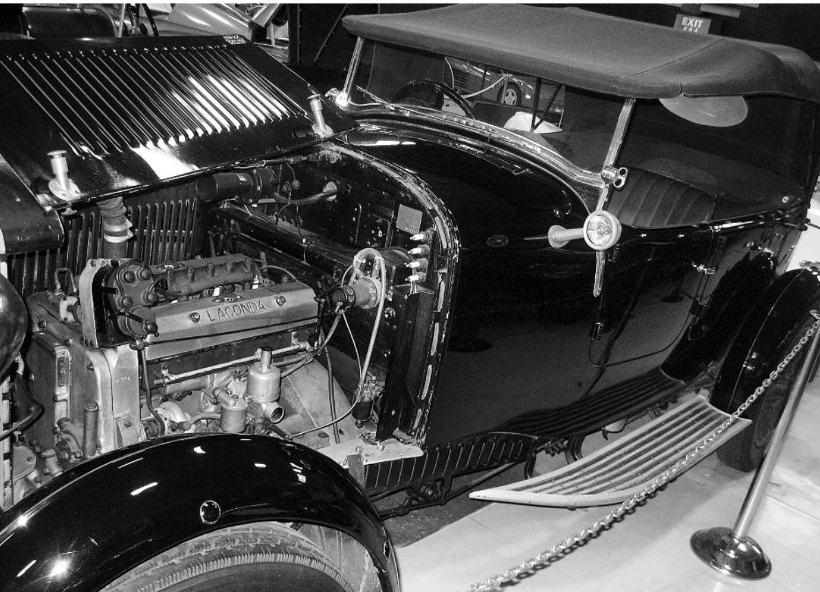
Above: 1931 Lagonda “Low Chassis, Two-Liter” 60 hp touring car with hemispherical cylinder heads. The front cycle fenders turned with the wheels, and the body was fabric-over-wood. Lagondas were known as the “poor-man’s Bentley.”
