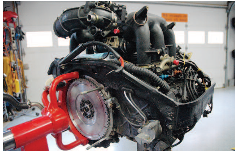
Engine was stripped of all unnecessary pieces. Stock flywheel was replaced with a conversion unit from Patrick Motorsports. The original plan was a hot race engine built from a 2.7-liter starting point. A couple of kids underfoot made safety become the driving factor and switching to a 3.6 engine reduced the mental conflict whenever a safer but heavier option was considered.
