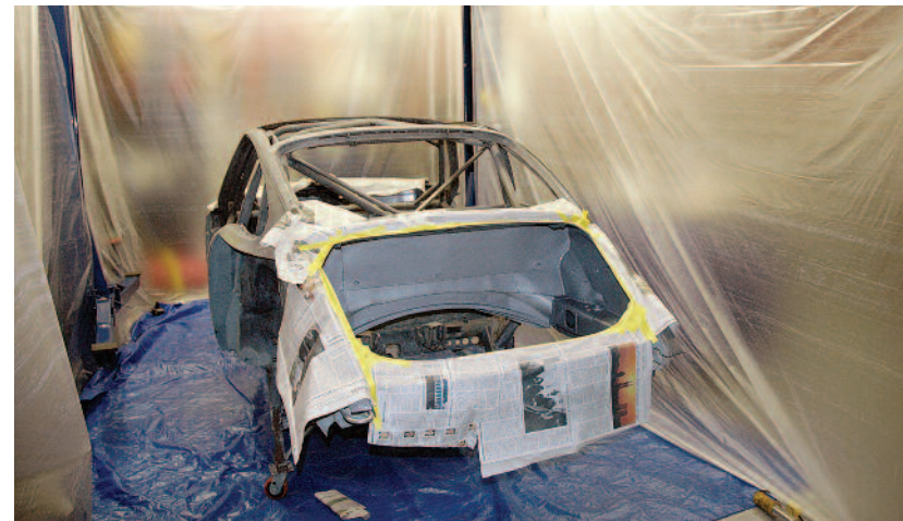
Mickelwait made his own paint both using string and thin plastic drop-clothes. Ventilation was with two box fans with filters taped to them. Body used a lot of masking and steps. Painting a roll cage and complete interior requires more body joints than humans come with, he says.
