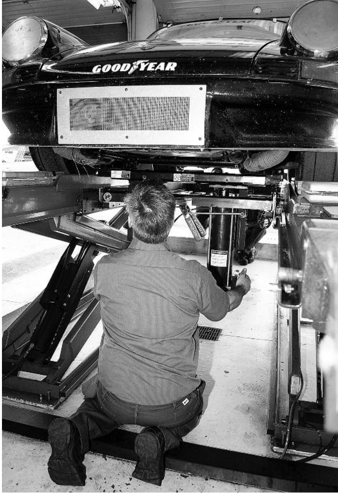
Above: Chapman rolls the car onto the scales from the wooden blocks. Then he jostles the car up and down to settle the car onto its suspension. Empty, Siciliano's 911 weighed 2,100 lbs.
