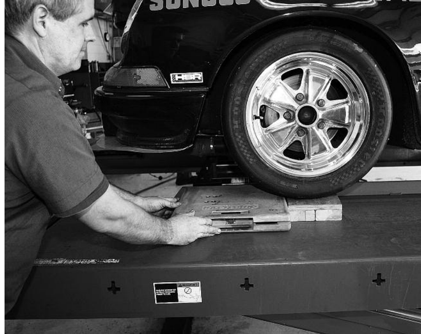
Above: Chapman rolls the car onto the scales from the wooden blocks. Then he jostles the car up and down to settle the car onto its suspension. Empty, Siciliano's 911 weighed 2,100 lbs.
