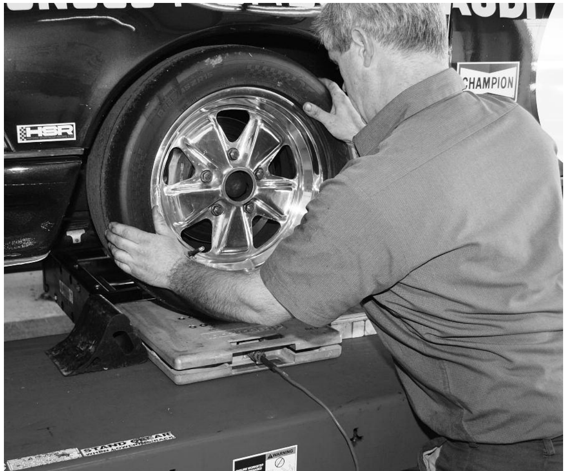
Left: The Hunter lift has built in jacks that enable Chapman to raise the car in order to set it on the wood blocks. The car is then rolled onto the scales. Chapman says that 911s need a forward rake of 1 degree. He sets up the corner weights according to what the driver wants. Drivers can make small adjustments later, he says, through sway bar adjustments and tire pressures.
