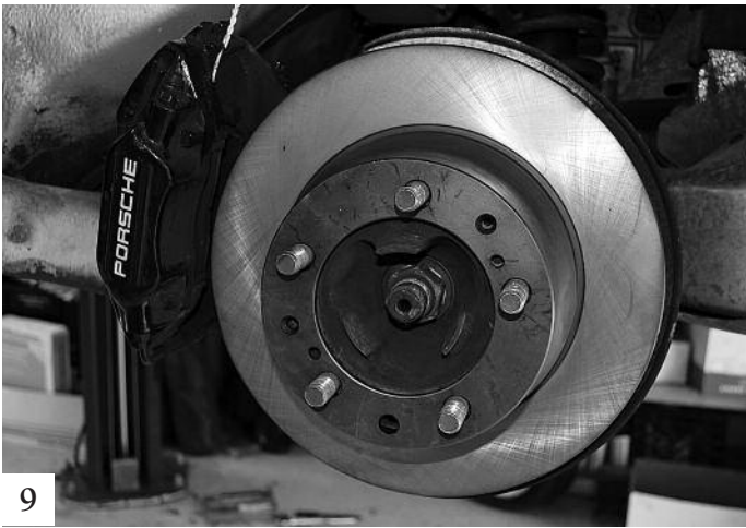
No. 9 The new rotor installed. Securing the rotor to the hub with the two screws is optional. Especially if the rotors have been removed previously, these screws might be missing anyhow.
