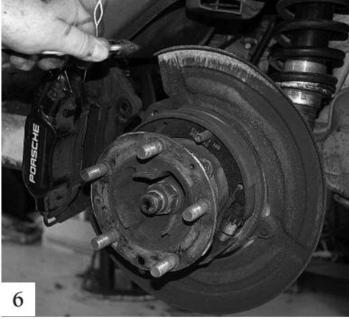
No. 6: Using compressed air, blow out accumulated dust and debris.
