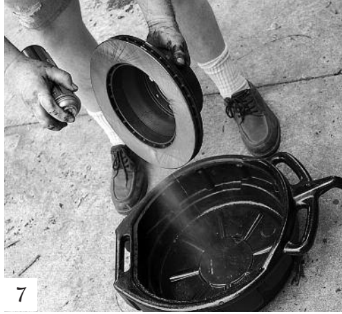
No. 7: Clean both sides of the rotors with brake cleaner before installation.
