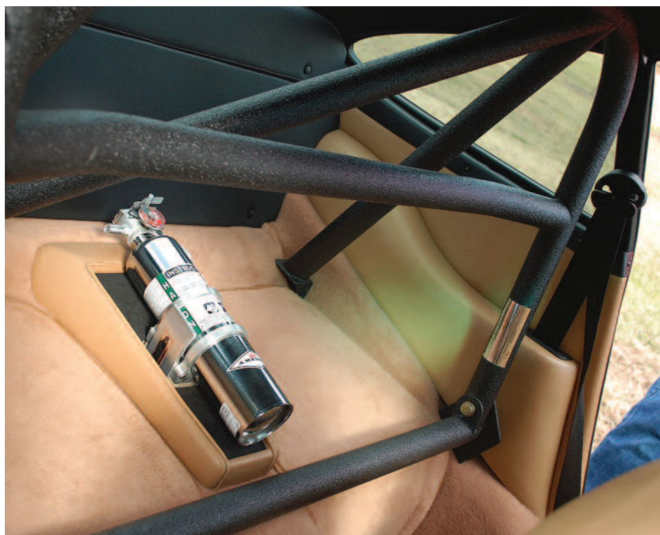
Above and right: The custom mount for the fire extinguisher (seen at right) was made by Bockelmann (above) using corrugated cardboard for a mockup advancing to carved MDF, which was then covered in matching upholstery by Robert Appel. The rollbar, right, was covered in truck bed liner material.
