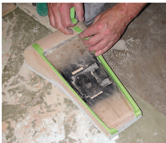
Above and right: The custom mount for the fire extinguisher (seen at right) was made by Bockelmann (above) using corrugated cardboard for a mockup advancing to carved MDF, which was then covered in matching upholstery by Robert Appel. The rollbar, right, was covered in truck bed liner material.
