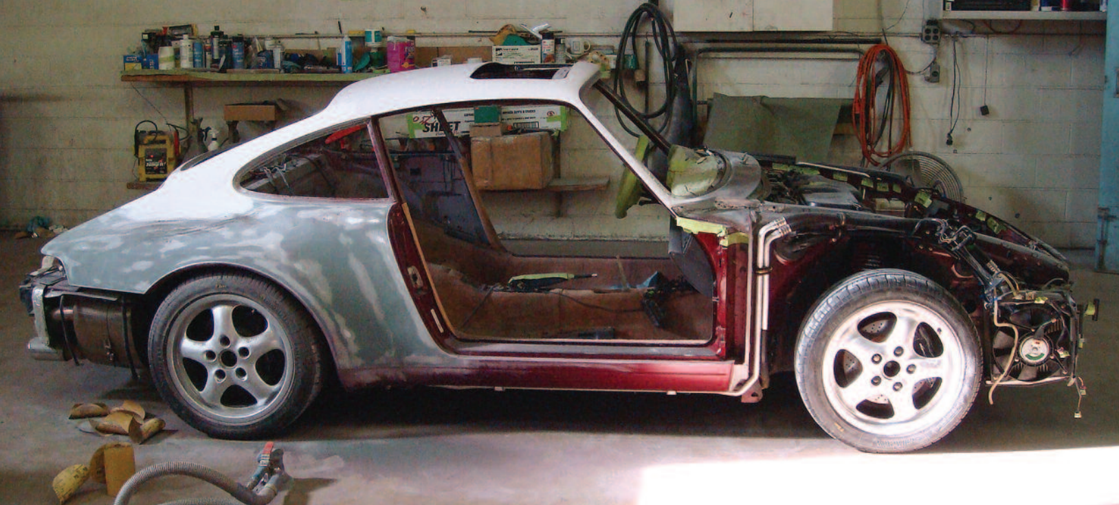
Above: The car as it sat after a new roof was welded on and the body was stripped prior to painting.
