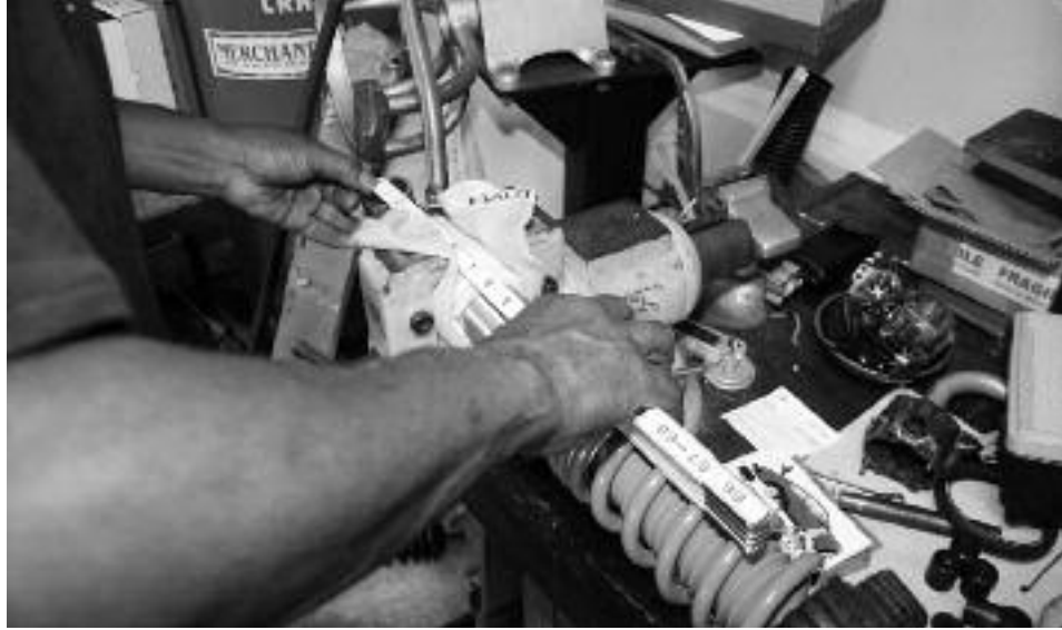
Bilstein PS9 shock absorbers come with instructions on how to set the spring adjuster height as measured from the center of the bolt hole to the adjuster.
