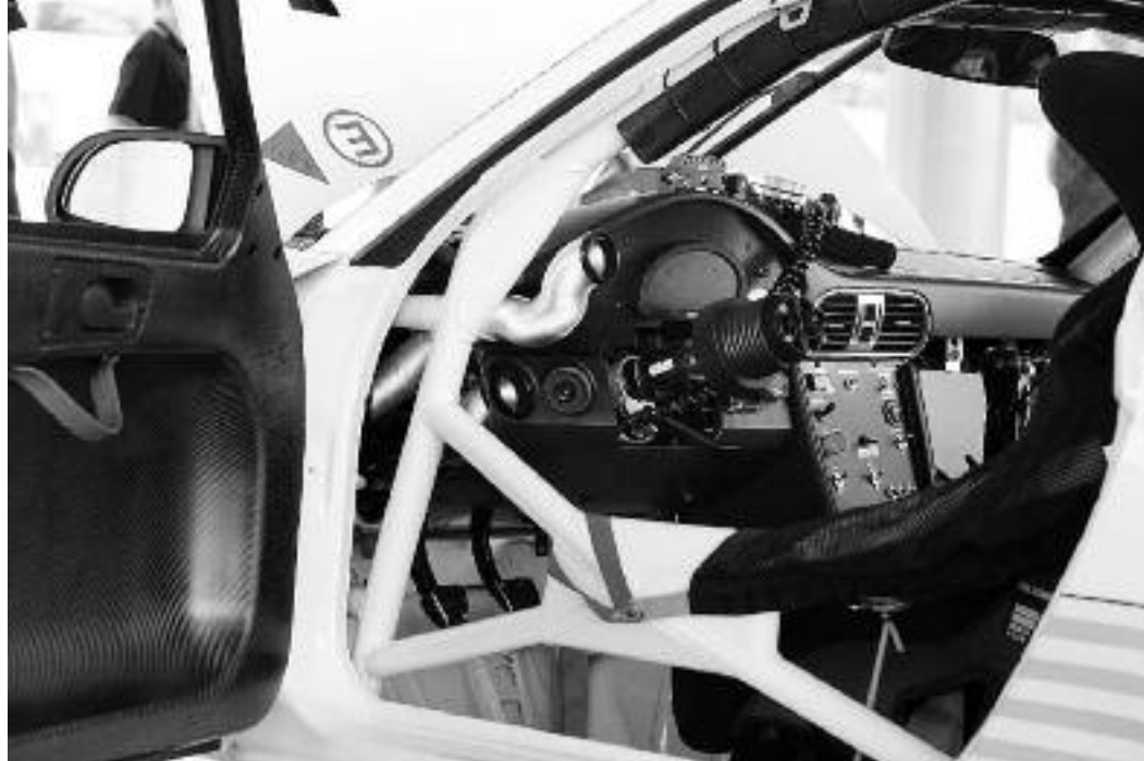
The cockpit area of the GT3 Cup car is complete with all gauges, removable steering wheel, camera data logger. The cars also have adjustable ABS and a sequential shifter.
