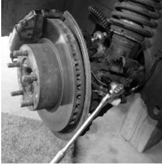
The front shocks are held to the hub by two 10mm Allen bolts. Do not use an impact wrench on these.
