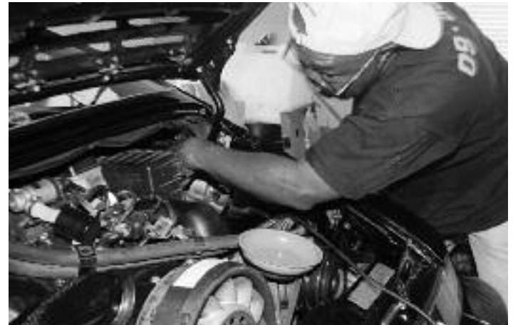
Jennings removes the three 13mm nuts from the passenger side rear shock absorber. Removing the air filter assembly aids in access, but the nuts are still awkward to reach.
