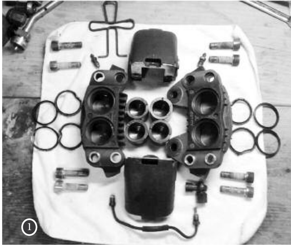
The caliper disassembled into all its component parts.
