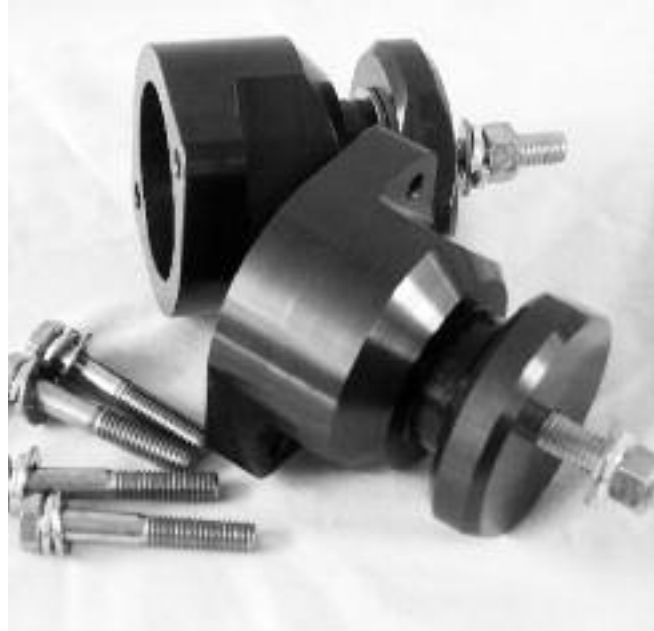
The old engine mounts (left) don't compare favorably to the new ones (right).
