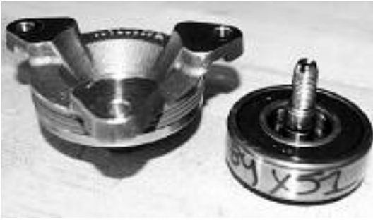
A deep flange will be a single-row bearing (above). A shallow flange (right) will be a dual-row bearing.
