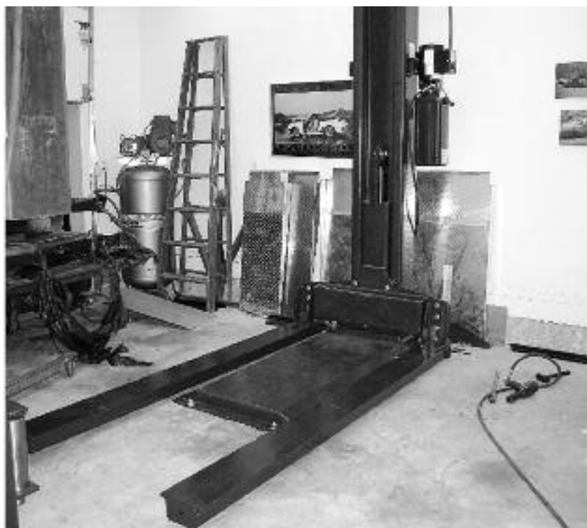
Below: The single-post lift is bolted down and working perfectly.
