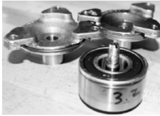
A deep flange will be a single-row bearing (above). A shallow flange (right) will be a dual-row bearing.
