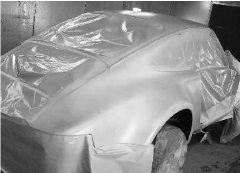
Center: The tub in the paint booth after being primed. You can note evidence of the guide coat having been applied. Guide coats are a thin misting of a contrasting color of paint—in this example, black—that help identify high and low spots to be corrected in the body during blocking and sanding before the final coats of color are applied.
