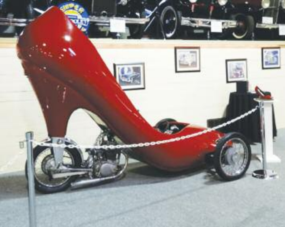
Above: The Red Slipper vehicle built on a three-wheel motorcycle layout featuring a Honda 350cc twin-cylinder engine.
