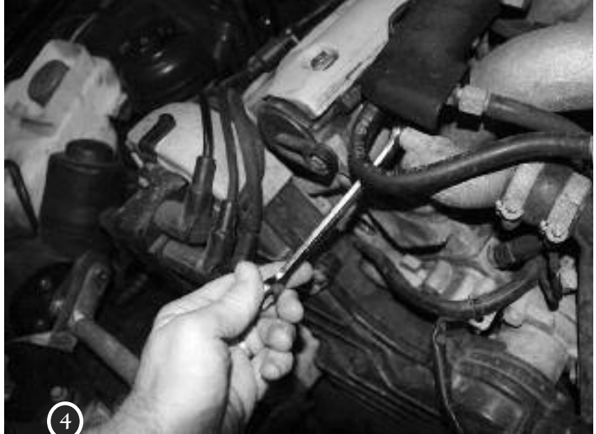
Above: Burp the cooling system of air by loosening the bleed screw.
